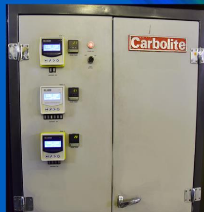
MET-Therm Programmers used in the MASTER/SLAVE configuration in Carbolite High Temperature Furnace with 3 zones (1 MASTER/2 SLAVES)
